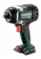
The SSW 18 LTX 800 BL by Metabo provides a maximum tightening torque of 590 ft-lbs., breakaway torque of 885 ft-lbs., no-load speed of 2,575 rpm, and impact rate of 3,300 BPM – all driven by a ½" square drive with friction ring. It is available as a bare tool (602403840), or as a 2x8.0 LiHD battery kit complete with ASC 55 charger (US602403620). Both versions come standard with belt hook and metaBOX 145 stackable carrying case.
