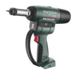
The 18V Brushless Rivet Nut Gun by Metabo has a quickchange mandrel system that can rivet up to M10 in aluminum, M8 in steel and M6 in stainless steel. It includes an easy setting force adjustment with 99 values and 10 memory settings. In addition, it has an autoreverse feature that automatically resets the tool for quick reload.
