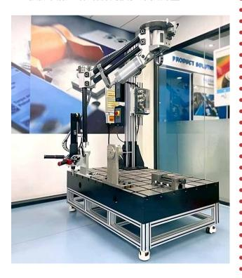
This assembly simulation system by Bossard (Shanghai) is equipped with a robotic arm that simulates actual assembly conditions to obtain the torque and angle relationships of the assembly setup, thus verifying the accuracy of the assembly process.
