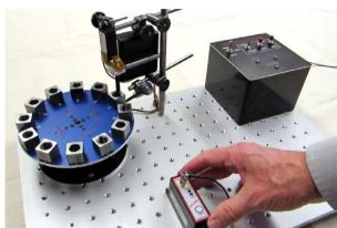
The ThreadChecker by Kaman Precision Products is a teachable eddy current inspection tool, widely used for thread detection, plating presence, and absence of heat treatment, as examples. Any physical property difference that relates to material conductivity is readily detected. The ThreadChecker is ideal for use in any automated inspection process in manufacturing.
