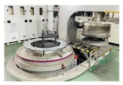
MIRDC developed a surface treating machine to handle anti-corrosion and surface hardening treatment for stainless steel parts, providing solutions to deficient stainless steel hardness, weakened corrosion resistance and inability of mass-production. The machine can make for stainless steel surface hardness up to over HV1,200, much higher than with carbon steel and without undermining corrosion resistance.
