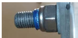
Fig.5. Fast assembly speed nylon insert separation.
