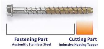
"300 series austenitic steel features exceptional anti-corrosion. While used outdoors, they reveal greatly increased service life and avoid security issues related to corrosion-incurred screw anchor failure, especially in highly corrosive environments. Tips made of harden-able carbon steel are used as lead threads during fastening to avoid unsuccessful fastening of stainless steel bodies due to material properties," says Sheh Kai Manager Barry Tsai.
