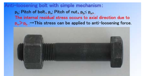
Fig. 9.9 The anti-loosening bolt with a single nut (This mechanism can be applied to an embedded bolt)
