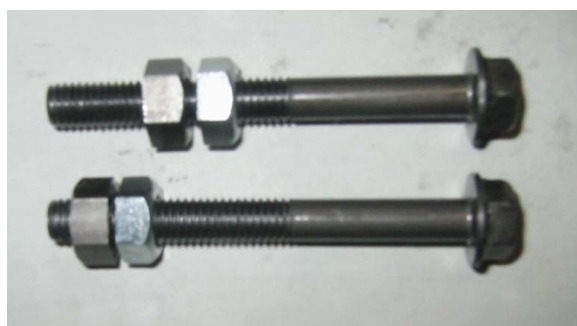
Fig. 9.6 An outer appearance of the double thread bolt
