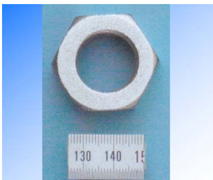
Fig. 9.11 Shot peening treatment at the end of nut
