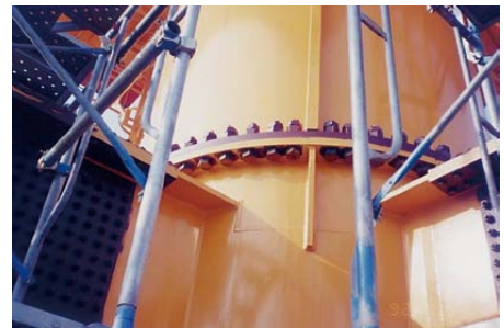
Fig.8.18 Setup of the CD bolts to the mast of a climbing crane
