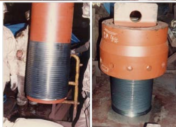
Fig. 8.1 Tie rod of a rolling mill ( \phi 475 \times 13,975 mm in length)
