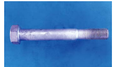
Fig. 8.5 The CD bolt of steel tower for power supply across Oto-channel in Kyushu power company
