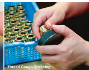
Thread Gauge Checking
