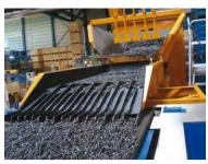
SKAKO VIBRATION - furnace feeding systems are a very important part of many industrial processes e.g. for the automatic and weight guaranteed belt- and tempering furnaces. Controlled, automatic and weight guaranteed feeding of bulk material ensures a steady product quality, and optimized efficiency of the downstream equipment of all kinds of bulk material.
