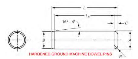
10 times better than the tolerance of the part being measured. In other words, since dowel pins have a .0002" tolerance, the instrument used to measure that precise should have a resolution of .000020" (Twenty millionths of an inch). This practice is suggested so that you have enough increments to be able to clearly determine if the measurement is inside or outside of the required specification.
