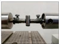
The most practical instrument set up to measure dowel pins accurately is what most people call a bench comparator or super-mic. Essentially a highly accurate, rigid, linear measuring machine with a digital readout and the ability to regulate measurement pressure similar to the unit pictured below.
