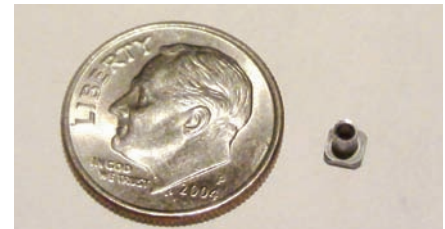
Figure 4: Square Head with Internal Back Extruded Shank
