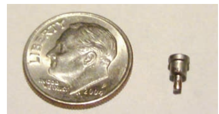
Figure 5: Shoulder Screw for Computer (Blank-Not Threaded Yet)
