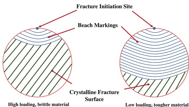
**Figure One** Illustration of a Typical Fatigue Failure Fracture Surface
