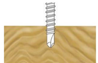
Figure 1. A cutting blade sends the waste material back up the body of the screw
