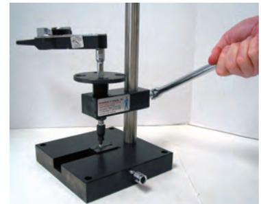
4. The torque wrench is firmly engaged in the upper end of the rotating shaft's female square recess. The wrench's indicator is set to "zero" before any torque is exerted on the wrench.
