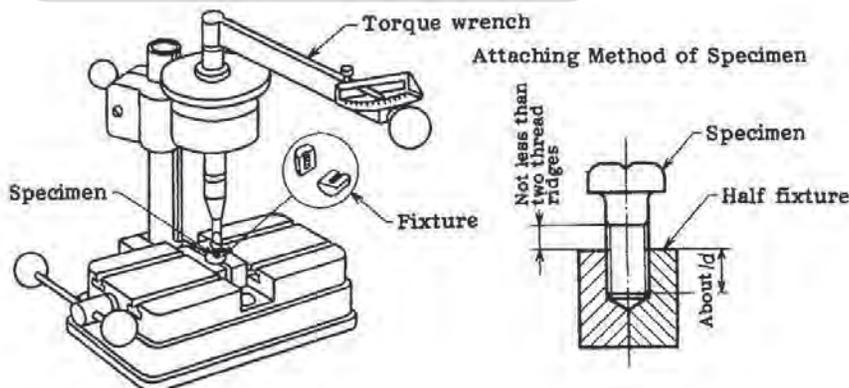
Although these standards do not always agree on the Torsional Strength values for a particular size fastener, fortunately for screw suppliers there is agreement regarding the testing apparatus and the procedure. The typical torsional strength testing apparatus is illustrated below.
