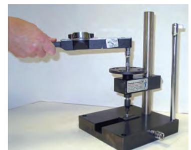
5. A smooth continuous torque is applied by the torque wrench until the screw twists into two separate pieces. The torsional strength of the tested screw is the highest torque value observed on the wrench at any point during the test.
