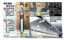
On April 10 Australian anchor system manufacturer Hilti warned its contractor that the use of 3 defective HSL-3 M24 series of anchors in Hong Kong High-Speed Rail produced during May 2011 through August 2013 may reduce the tension capacity largely by 60-70% though without influencing the shear strength.
