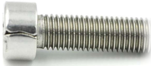
Figure 5: Cracked Head from Wire Seam
