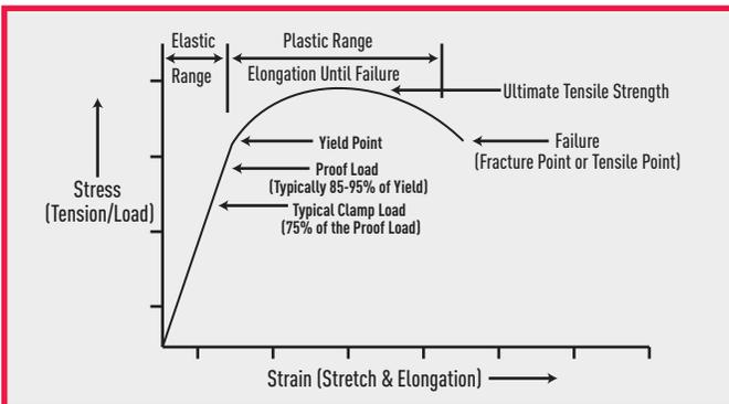
Figure 2: Load versus Elongation
