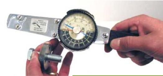
Observe the maximum torque value on torque wrench
