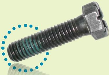
These bolts were replaced in the clutch and torqued into a tapped hole to the specifications given in the manual. The vehicle was placed in service, where a short time later, the bolts had head failures. No one thought to think that the epoxy would cause the failure.
