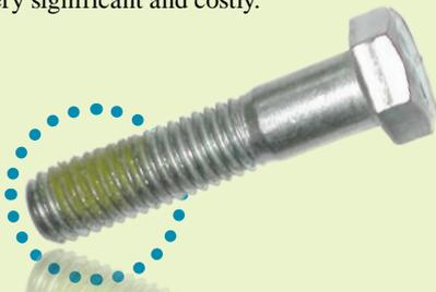
These epoxy type of locking aides are very good if used properly. Most users will not employ a torque wrench to tighten their fasteners, so these epoxy coated fasteners will work well. However, caution must be observed when using any air impact assembly tools, as these fasteners will not have sufficient friction to cause these tools to stall and the fasteners will be either stretched into yield or have their threads stripped.
