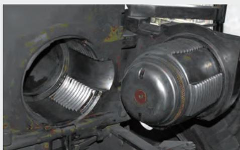
Figure 2. Interrupted thread used on a military gun. [Image credit: public domain]
