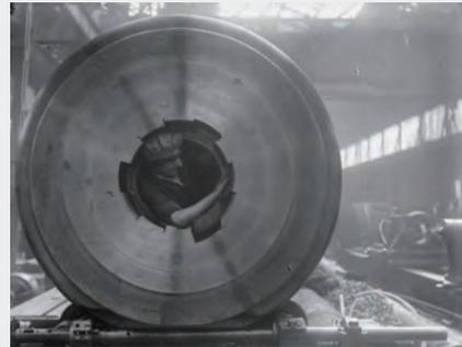
Figure 3. Worker cleaning the threads of a Welin breach on a 15 inch gun. [Image credit: public domain]
