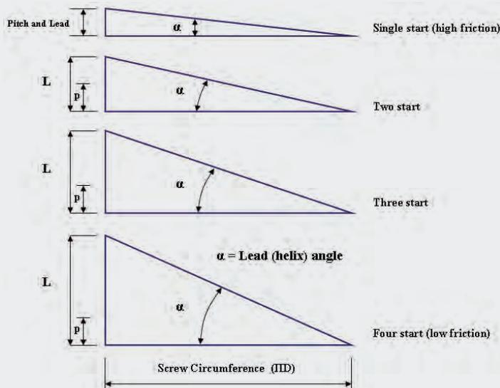
Figure 1. Relationship between Pitch and Lead.
