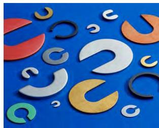
Boker's, a manufacturer of precision metal stampings, washers, spacers and shims, offers a wide variety of custom C-washers to its customers. C-washers obtain their name for being in the shape of a "C" as they have a slot cut from the center to the perimeter allowing the washer to be removed, replaced or inserted without completely removing the fasteners.
