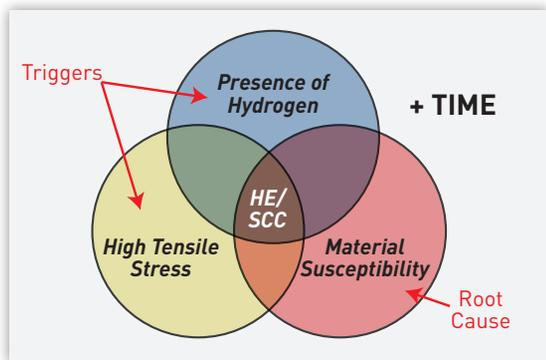
*Figure 1: Required Parameters for a Hydrogen Embrittlement Failure*
