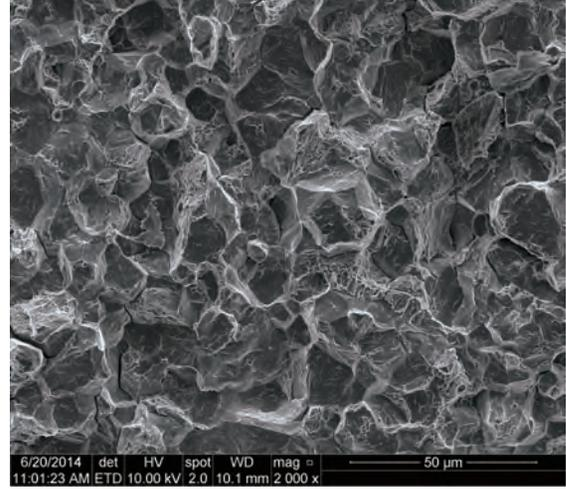
*Scanning Electron Microscope Image of a Hydrogen Embrittlement Failure Showing the Characteristic Intergranular Brittle Fracture Morphology (used with permission of SV Brahimi)*
