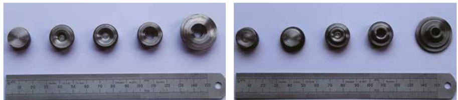
Figure 1. Production sequence for valve spring retainer (courtesy KMS)
